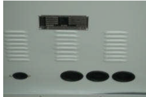
LAN/P.C - External connection – lower rear left case on a 3 Phase PropSava.
